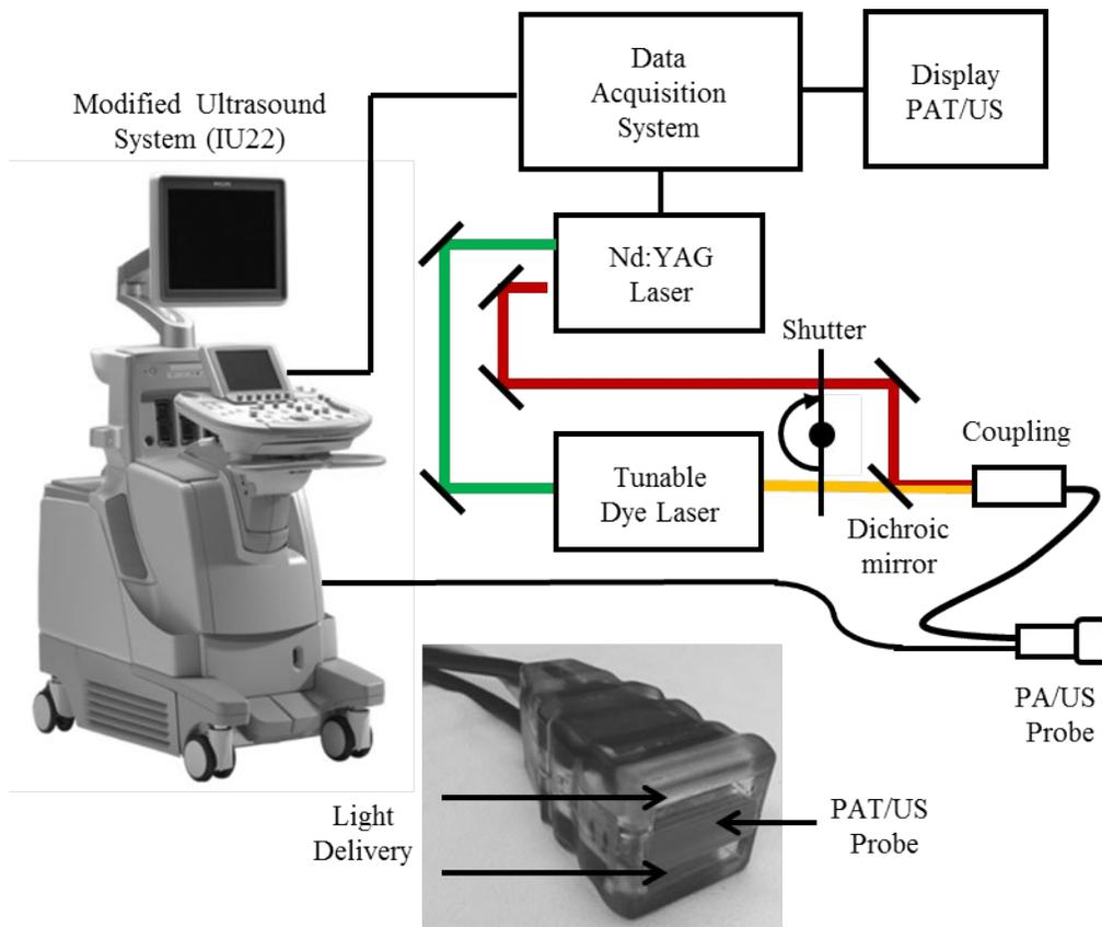
Figure 2. Schematic of the dual-modality photoacoustic and ultrasound imaging system and improved ultrasonic transducer design. The transducer features a flat surface for light delivery and fiber bundles integrated into the transducer housing for easier handling.
